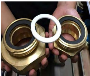
ETHANE & ETHYLENE TANK CONNECTION WITH PTFE TEFLON GASKETS
