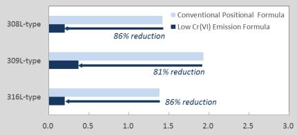
Hexavalent Chromium Emission Rate in Welding at 200A with 75%Ar-25%CO<sub>2</sub> (mg/min.)
