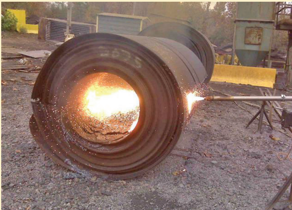
After switching from propane to propylene, the user increased cut speeds on this 32-inch steel coil from 4 inches per minute to 10, while realizing a 60 percent improvement in production and costs.
