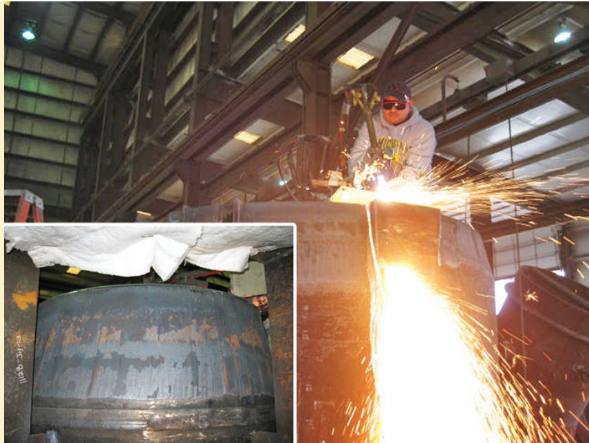
With Gas Innovations and propylene, the distributor helped the end-user achieve a 27-inch, 75-degree bevel cut on 5 \frac{3}{4} -inch 516 grade steel. At bottom left, the finished, clean bevel, ready to weld.
