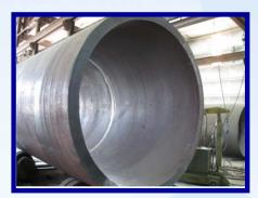
98" Dia. VESSEL 176 ¼" Long 5 ¾" Thick 516 grade steel 75 ° BEVEL
