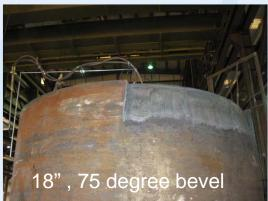
Before using Oxweld torch and two heating heads. could only cut 8" with Propane. With the Gas Innovations torch set at 30 PSI Propylene, 25 Preheat Oxygen and 150 PSI cutting Oxygen. This equals approximately 110 lbs fuel gas/hr and 5,000 cuft of Oxygen / hour.
