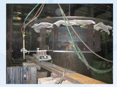
Torch set up for 32" straight cut: Propylene 35 PSI Preheat Oxygen 28 psi Cutting Oxygen 180 psi
