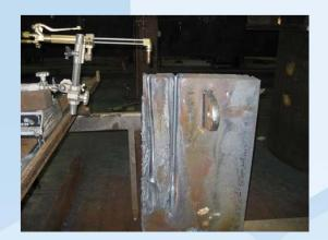
Hand Torch test set-up for 32" cut. Could only cut 22" because of 90 degree head looses cutting oxygen velocity.
