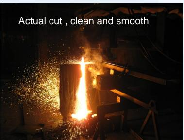
Below Torch was set at a 10 degree angle to get a clean start. Stopped cut prior to completion show length of cut.
