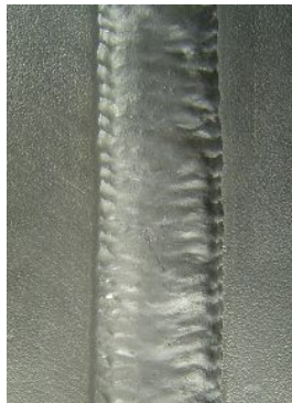
Bead appearance and macrostructure of butt joint for DW-N625 (3G)
