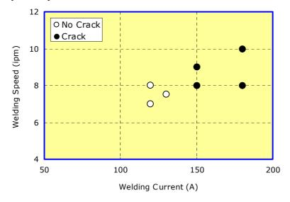
The weld metal composition of DW-310 is of the 25%Cr-20%Ni type, and has a fully austenitic structure. Due to the nature of austenitic materials, great care must be taken to prevent cracking. It is recommended that DW-310 be used with the welding current of 150A or less. In first pass welding of a narrow V-groove joint or large stress concentrated joint, a welding current of 140Ams or less is recommended. This will increase the weldments crack resistibility.
