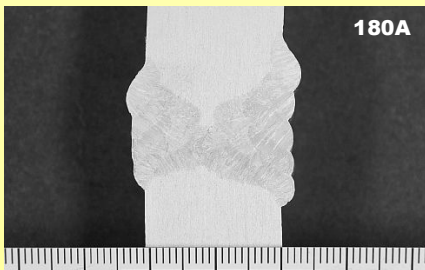
Macrostructure of butt joint (2G)
