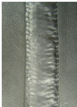
Bead appearance and macrostructure of butt joint for DW-N625 (3G)
