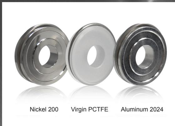
Manufacturers of the highest quality Ultra High Integrity Service (DISS) gaskets for CGA 632-728 connections. Available in Electropolished Nickel 200, Virgin PCTFE and Aluminum 2024. Produced in accordance with CGA V-1 standards. 100% visually inspected, ultrasonically DI cleaned, clean room packaged, labeled with processing batch number for traceability. Available from stock.
