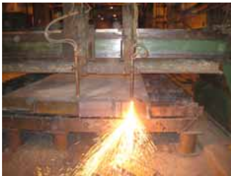
NEW OFSHX-6 PROPYLENE TIP, NO PREHEAT REQUIRED ON HIGH NICKEL 6.5" STEEL USING PROPYLENE
