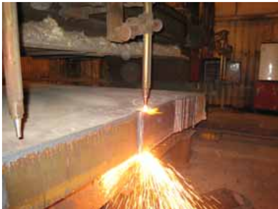
HIGH NICKEL STEEL CLEAN CUT WITH SQUARE CORNERS NO ROLL-OVER AND SLAG FREE CUTS
