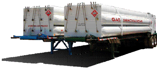
COMPRESSED GAS MODULES
