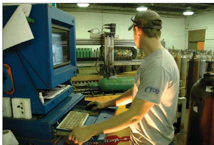
Ultrasonic Examination (UE) enables cylinders to be requalified without the need for valve removal or the discharging of cylinder contents.
