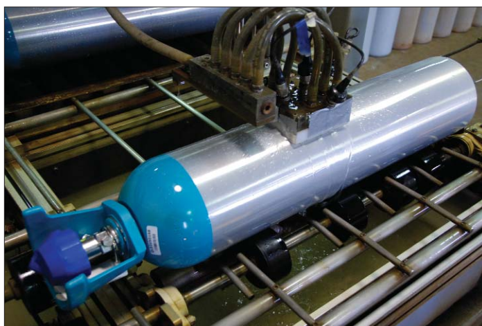
Ultrasonic Examination (UE) is gaining favor over traditional Hydrostatic Testing due to improved turnaround on TOS cylinders and longer valve life.
