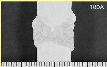
Macrostructure of butt joint (2G)
